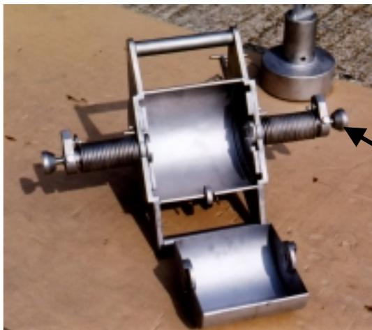
Please note that once you have pulled out the axial knobs, their position can be maintained by turning the knob so that a small cross pin engages with the housing. (See Fig. 4)
