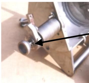
Cross pin pressing against housing, to retain the position of the axial knob.
