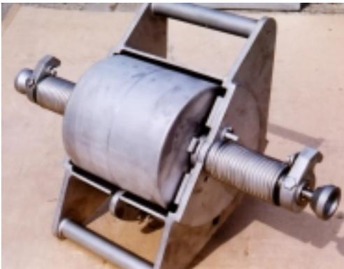
Similarly, on recovery, the bucket containing its sample can be removed for examination, by withdrawing the spring loaded pins and following the reverse procedure.
